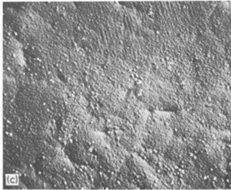
Figure 6 Etch features produced on \{100\} surface of a Ge-doped \langle 100 \rangle axis crystal etched for (a) 60 min in solution A–B at 60^\circ\text{C} , (b) 60 min in solution A–B at 60^\circ\text{C} and a further 40 sec in solution H, (c) 60 min in solution A–B at 60^\circ\text{C} and a further 100 sec in solution H.
